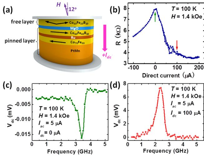
FIG. 1. Sample structure and ST-FMR spectra. (a) Schematic view of the MTJ nanopillar. (b) Resistance as a function of direct current  $I_{dc}$  applied to the MTJ. Arrows mark the direct current values at which ST-FMR measurements shown in (c) and (d) are made. (c) ST-FMR response curve  $V_{dc}(f)$  measured at  $I_{dc}=0 \mu\text{A}$ . (d) ST-FMR response curve measured at  $I_{dc}=100 \mu\text{A}$ .
